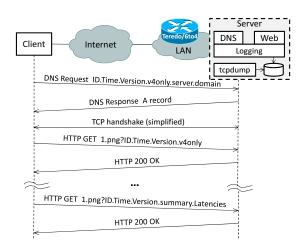
**Figure 2: Experimental setup**
